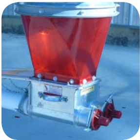
Anchor and Bearing Assembly; Translucent Boot Transition
