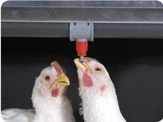
Chore-Time's breeder nipple has a shorter nipple pin and less lateral movement so both hens and roosters learn to drink directly under the nipple in a position that wastes less water.
