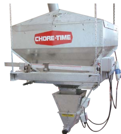
Suspended Feeder Line Hopper Scale
